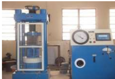
Figure 6. Test setup for Compressive Strength of Cube
