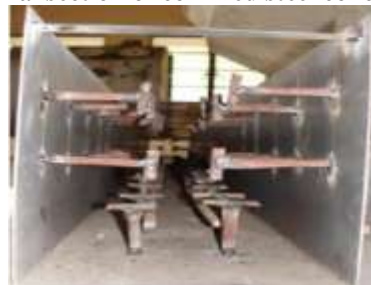
Figure 3. Cross section details of stud shear connector
